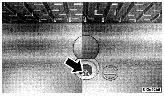
2. Engage the jack wrench extension to the spare tire winch through the hole in the floor.
